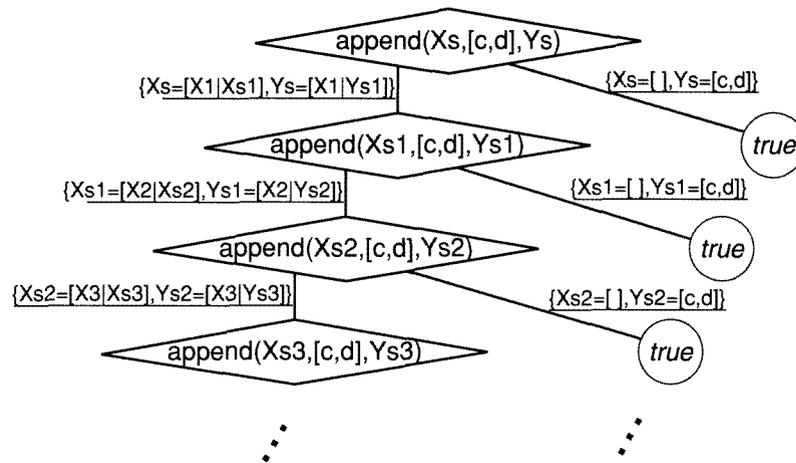
Figure 5.4 Search tree with an infinite branch
