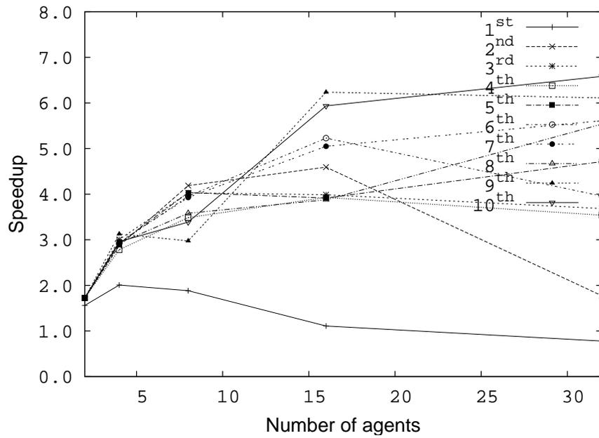
Figure 5.16: Speedups with stack set expansion for *Boyer*.
