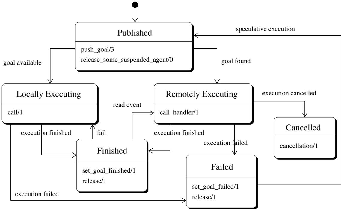
Figure 5.8: State diagram of a parallel goal.
