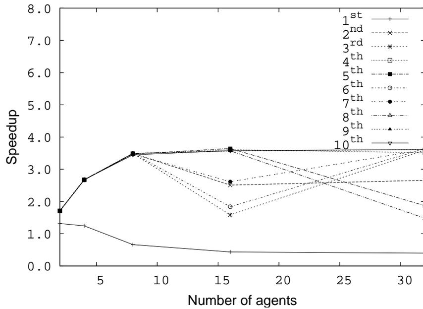
Figure 5.19: Speedups with stack set expansion for *QuickSort*.
