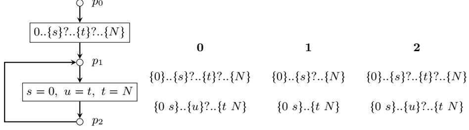
**Fig. 9.** Non-terminating analysis with array segmentations; column  $i$  shows the segmentation in round  $i$
