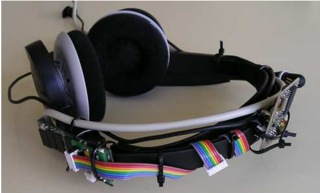
Figure 2: The sound spatializer prototype mounted on headphones. The compass is at the right of the image and the Gumstix board is at the bottom left.
