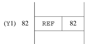
Then x2 is set to point to that stack slot (the value of A1); functor f/1 is pushed on the heap; and set\_value X2 pushes the value of x2 onto the heap:
