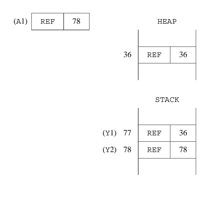
Line 3 sets A2 to the value of STACK[77]; that is,  $\langle \text{REF}, 36 \rangle$ .
