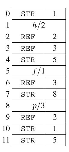
Representation of p(Z, h(Z, W), f(W)). starting at heap address 7.
