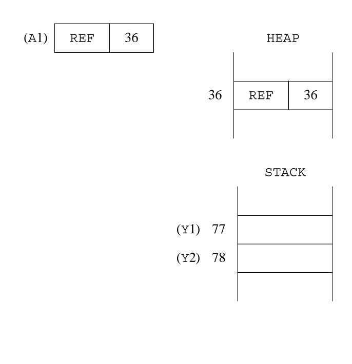
Line 1 sets STACK [77] to  $\langle \text{REF}, 36 \rangle$ , and Line 2 sets A1 (and STACK [78]) to  $\langle \text{REF}, 78 \rangle$ .
