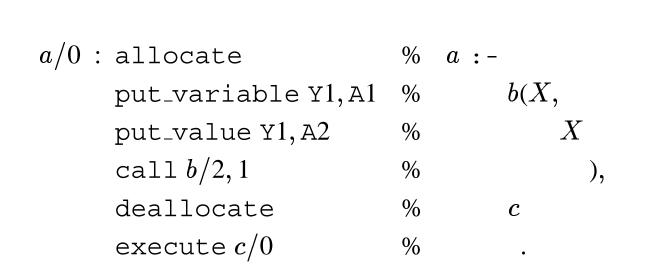
**Delayed trimming for** a := b(X, X), c.
